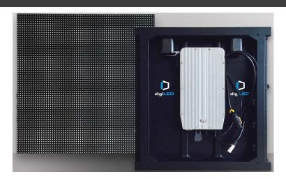
With a pixel pitch of 3.9mm, the digiLED DLPi3.9 LED Module offers designers a rugged, ultra-high resolution LED product. Black shell 3-in-1 SMD LEDs offer designers and content creators ultra-high definition images.
